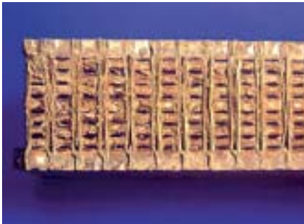
Poor performance caused by deposits
