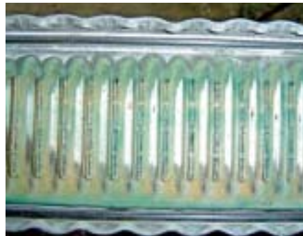
Furring due to the use of pure water (without coolant).
