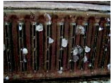
Additives cause reactions with the material and the coolant.
