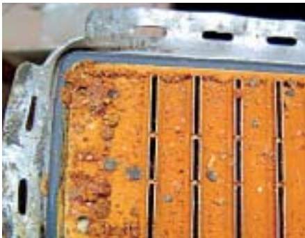
Deposits due to oil exiting stem from engine oil which gets into the coolant circuit due to a damaged cylinder head.
