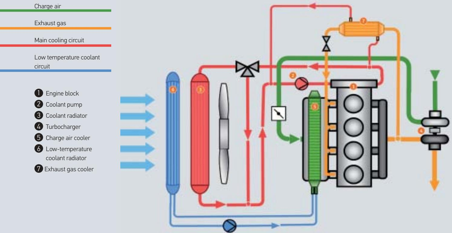
Schematic layout of the coolant circuits for a modern engine with cooled exhaust gas recirculation and an integrated, indirect charge air cooling system.
